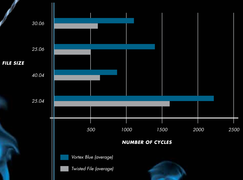
CYCLIC FATIGUE Vortex Blue vs. Twisted File
