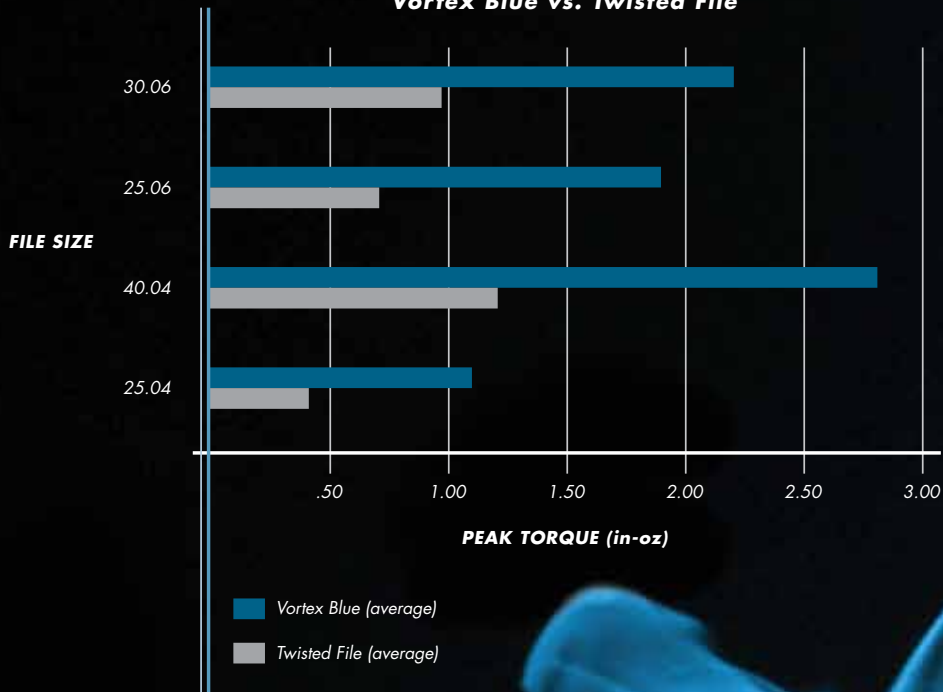
PEAK TORQUE Vortex Blue vs. Twisted File
